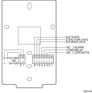
Fig. 50 - Indoor/Outdoor Air Quality (CO<sub>2</sub>) Sensor (33ZCSENCO2) - Typical Wiring Diagram
